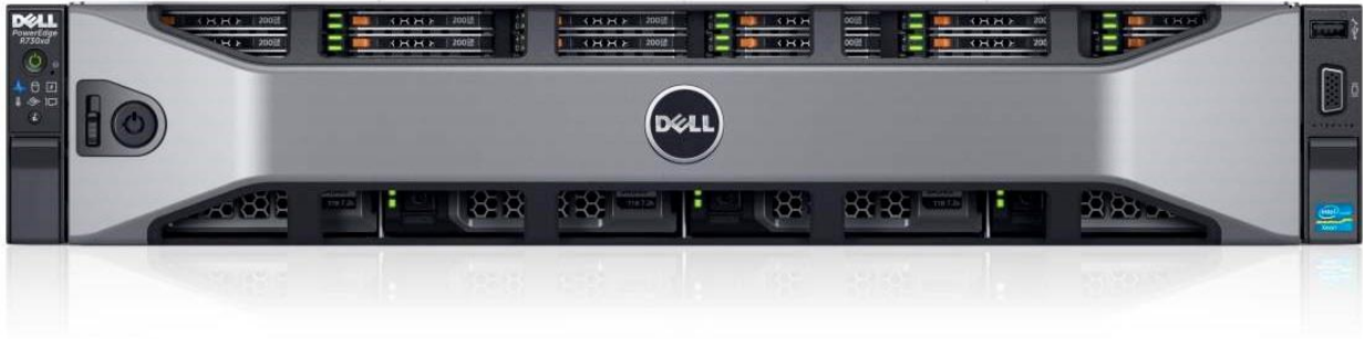
Figure 4. R730xd front view (8 x 3.5" plus 18 x 1.8" without bezel)
