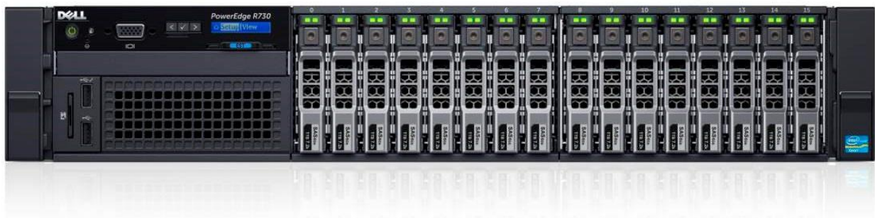
Figure 2. R730 front view (2.5" chassis without bezel)
