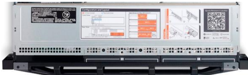
Figure 11. QRL on chassis
