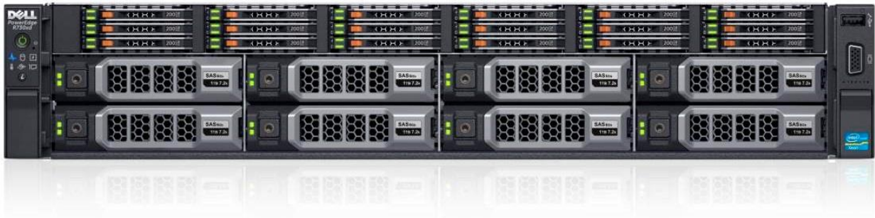
Figure 4. R730xd front view (8 x 3.5" plus 18 x 1.8" without bezel)
